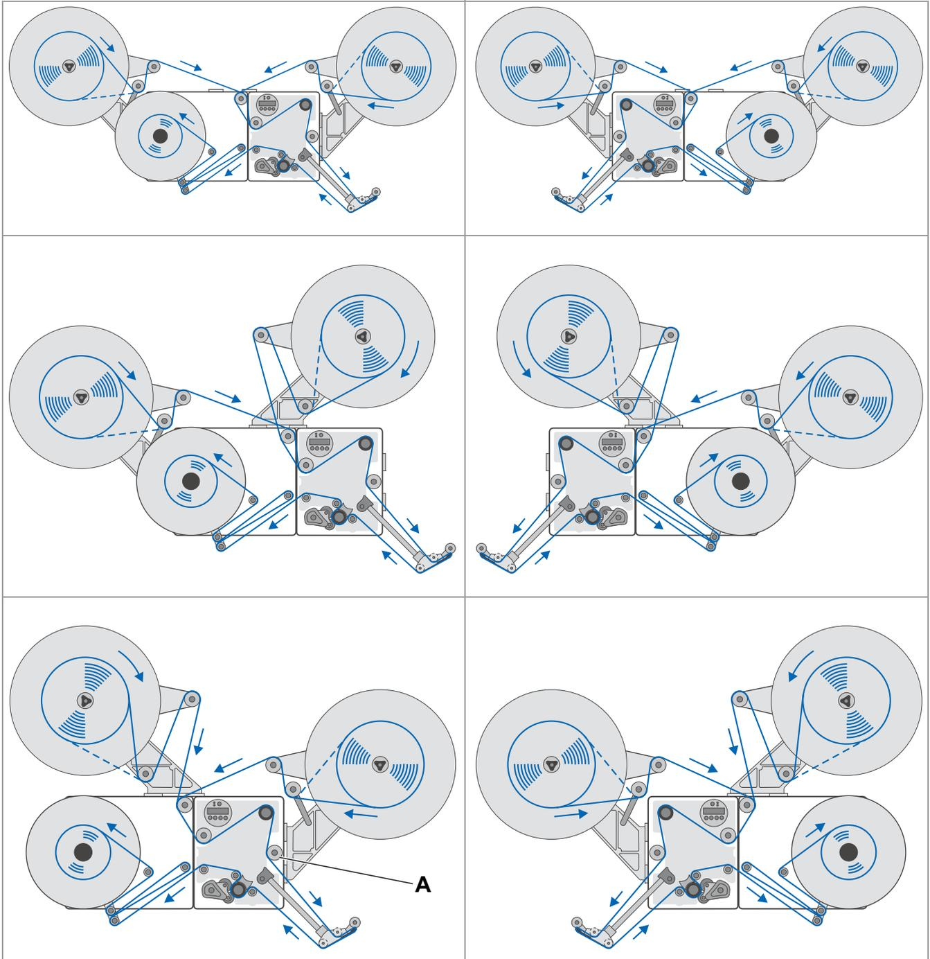
[40] Threading guide for ALS 30x with a 45° rotated dispensing edge (dotted line = roll with labels facing inwards).
