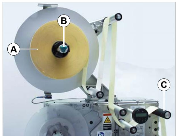
[38] Inserting the material roll.
