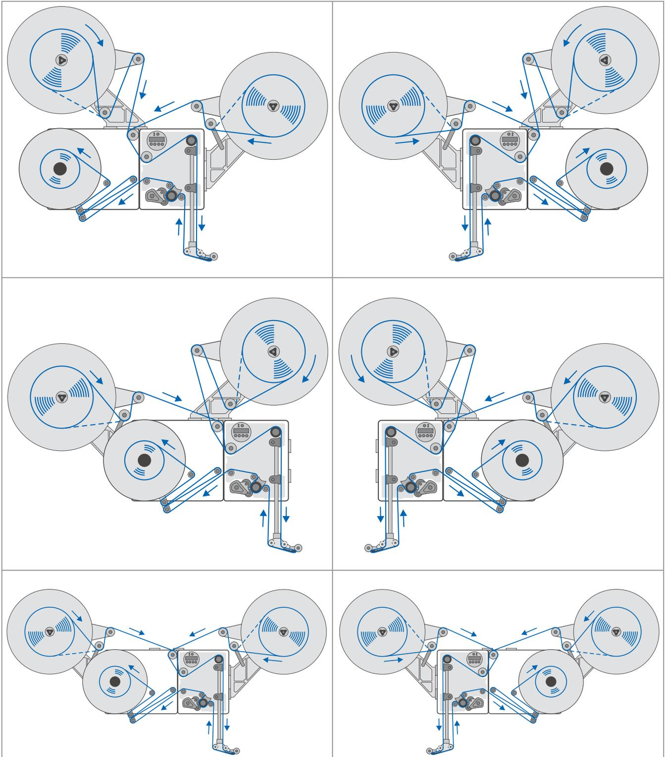
[39] Threading guide for ALS 30x (dotted line = roll with labels facing inwards).
