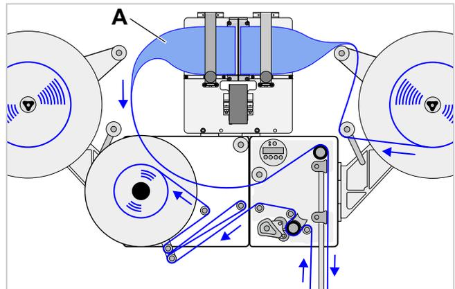
[50] Material end of the lefthand side label roll fixed at the splice unit.
