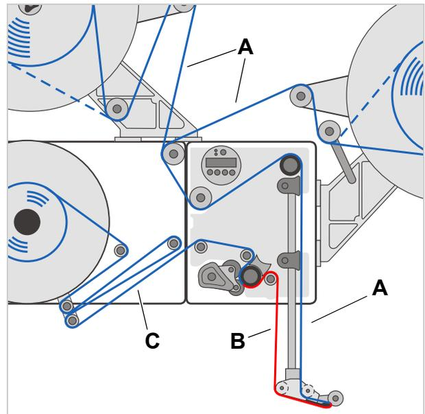
[66] Material tear off in sections A, B or C leads to different error messages.
