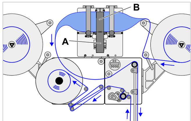
[51] Material ends bonded with adhesive tape.
