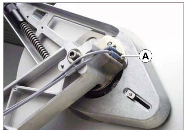
[35] Connectors (A) for internal OD-control at the unwinder.
