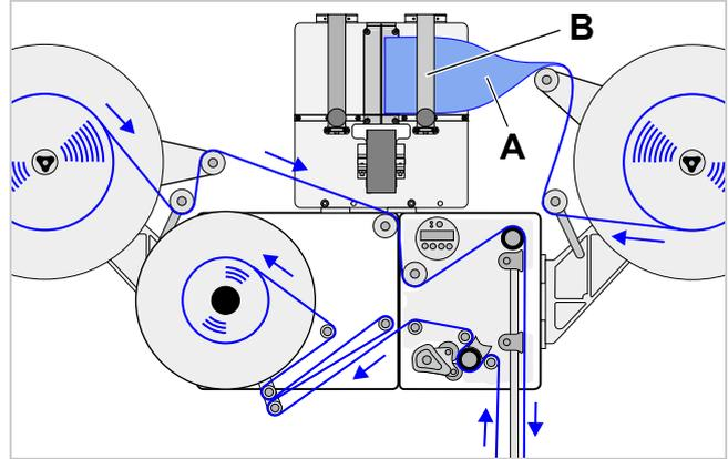
[49] Material end of the righthand side label roll fixed at the splice unit.
