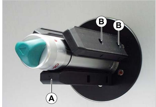
[52] Core adapter positions for a core diameter of 76.2 mm.
