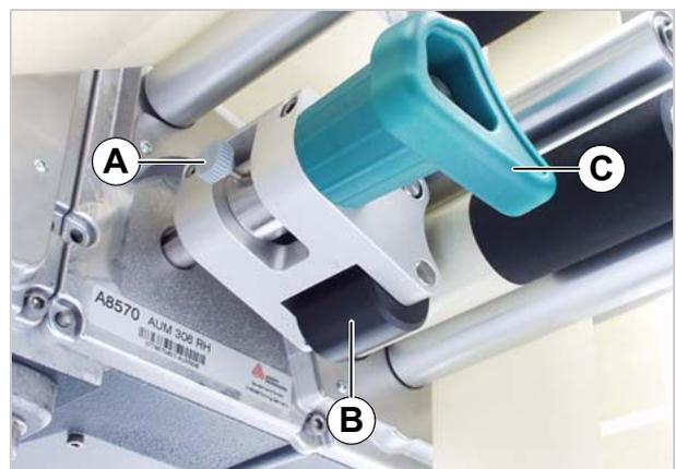
[54] Setting the position of the pressure roller (B).
